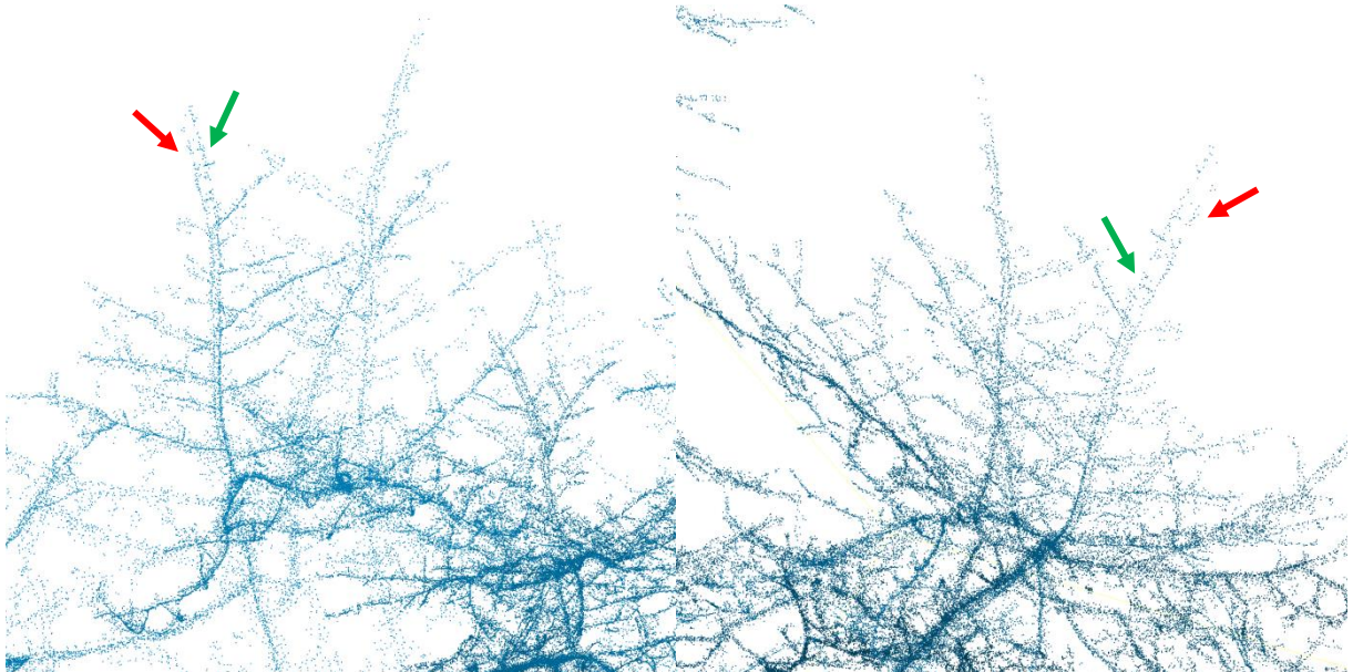
Fig. 14: Capture of the same twig of a C. betulus individual from different perspectives showing possible wind or registration artifacts. Red arrow pointing to either the falsely registered points or points recorded during wind.
