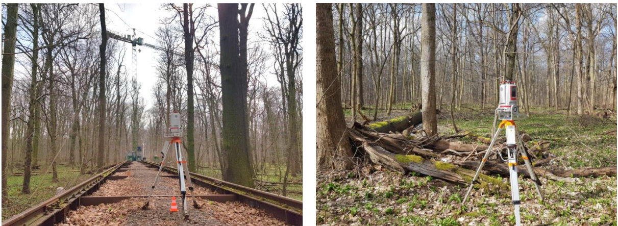
Fig. 2: Riegl VZ-400i in the field at the Leipzig Canopy Crane (LLC) Plot. Pictures provided by the project report [51].
